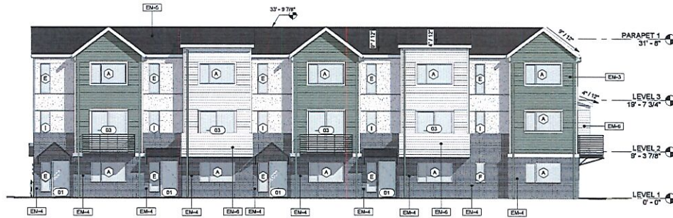
C1 BUILDING 1 NORTH ELEVATION 1/8" = 1'-0"
